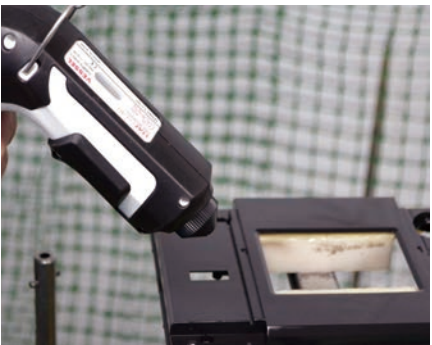
Static electricity removal of resin parts
