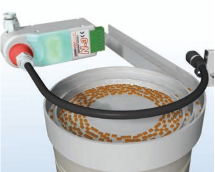
Vibratory bowl feeder (joint nozzle + shower tube)
